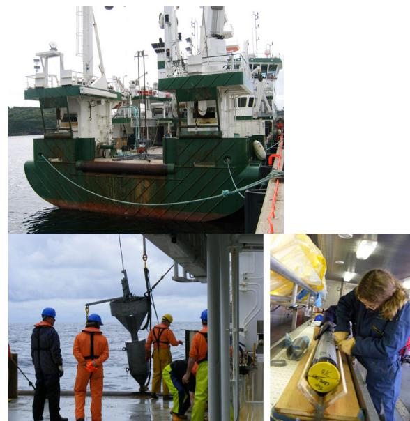
Figure 2 – Top: The Geological Survey of Ireland's vibrocorer (Geo-Corer 3000+6000) on the back deck of the R.V. Celtic Explorer. Left lower: The deployment of the piston corer Geo-Piston from the back deck. Right lower: Splitting one of the cores on board.
